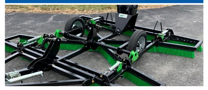
The CityBroom by GreensGroomer is a compact version of our GreensBroom for Scrub Seal and Chip Seal operations. The patent-pending design increases the effective surface area and improves brush angles which translates into significant performance gains. These designs control the emulsion into multiple directions, pushing coverage deep into the road profile, as much as 1-inch into the aggregate.
